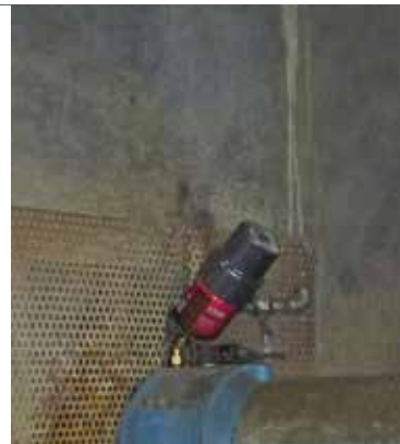
Lubrication system: perma STAR VARIO 120 cm 3
