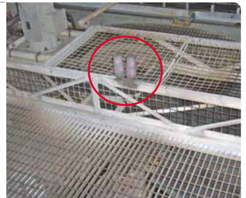
Lubrication system: 2 x perma STAR VARIO 120 cm 3
