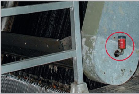
Screening: Lubrication of chain guide rollers
